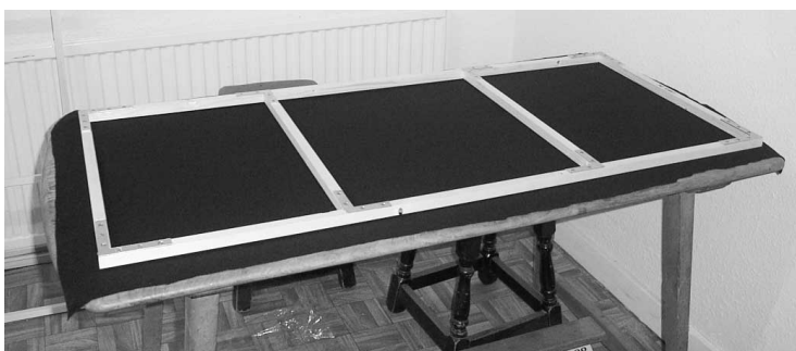
Cloth being attached to the frame.
